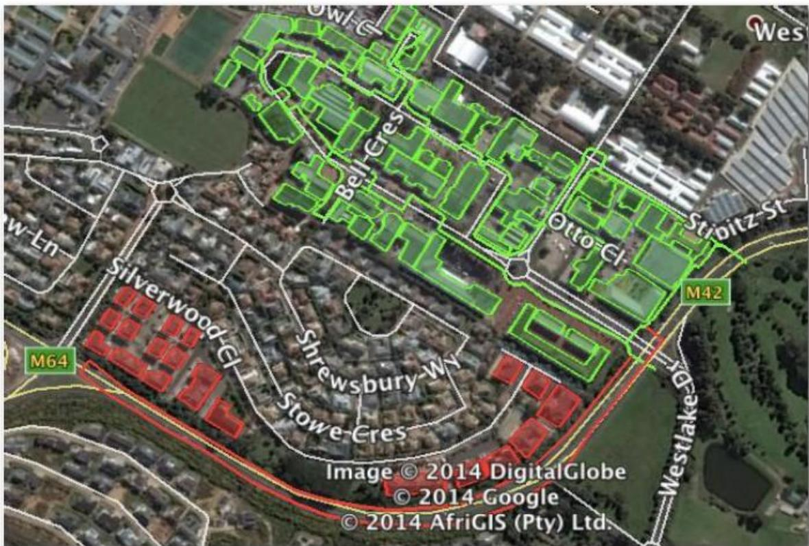
*Diagram showing the fibre optic ring network connecting all buildings in Steenberg Office Park with Westlake Business Park. The backbone network loops on both sides of Steenberg Road*
